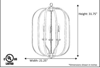
**ELECTRICAL REQUIREMENTS:** Fixture requires a grounded electrical supply line of 120 volts AC.
